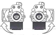
Housing rotated 1/4 turn to left — turn calibration screw 1/4 turn CLOCKWISE.
